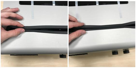
Once the gasket is loosened you can pull it off the machine.
