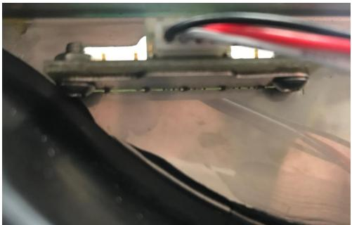
The cut out tab is cut with slots that simplify bending
