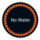
**No Water** warning is presented when the machine is unable to detect water at the start of the program.
