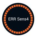
Warnings ERR Sens4 or ERR Sens5 indicate that the machine has failed to properly detect upper water level in the ultrasonic cleaning tank.
