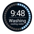
Degritter machine is using 300W of power for its ultrasonic cleaning. Most of this will be eventually converted to heat that will slowly raise the water temperature in the ultrasonic cleaning tank. Once the water temperature reaches 35 °C or 95 °F, the machine will insert a 3 min water cooling cycle into the washing program. This is done to prevent damage to the record from too high temperatures.
