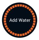
Add Water warning is displayed when there is not enough water in the removable water tank to fill the ultrasonic cleaning tank. Water will evaporate during washing and drying cycles and the water tank will need topping up.
