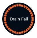
Drain Fail warning is presented when the machine is unable to verify that the ultrasonic cleaning tank has been properly emptied.
